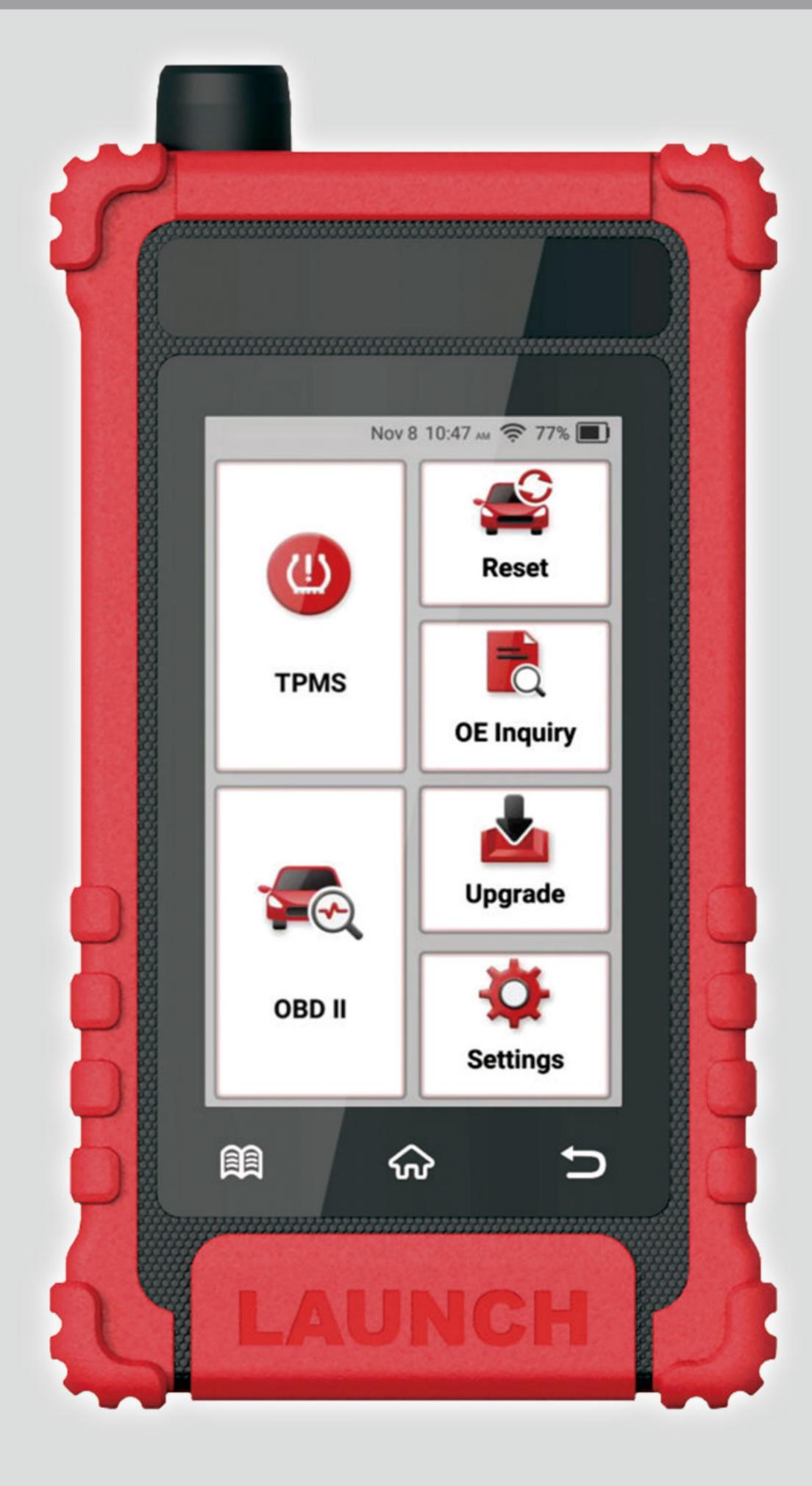
The 511S TPMS tool can activate, read and relearn all known sensors on the market. It can program LAUNCH TPMS sensors for unlimited times to replace OE sensors. The sensor data can be read instantly and accurately, including sensor ID, tire pressure, tire temperature, battery status, etc.
